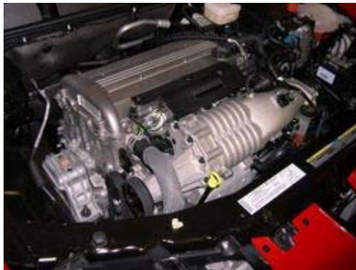
An Eaton MP62 Roots-type supercharger is visible at the front of this Ecotec LSJ engine in a 2006 Saturn Ion Red Line . Lysholm screw rotors. Note the complex shape of each rotor which must run at high speed and with close tolerances. This makes this type of supercharger quite expensive. (This unit has been blued to show close contact areas.)
