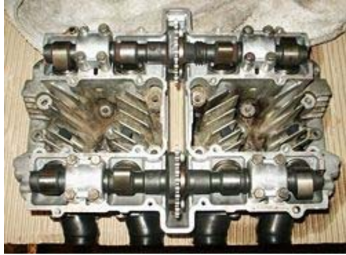
Overhead view of Suzuki GS550 head showing dual camshafts and drive sprockets.
