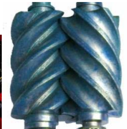
An Eaton MP62 Roots-type supercharger is visible at the front of this Ecotec LSJ engine in a 2006 Saturn Ion Red Line . Lysholm screw rotors. Note the complex shape of each rotor which must run at high speed and with close tolerances. This makes this type of supercharger quite expensive. (This unit has been blued to show close contact areas.)
